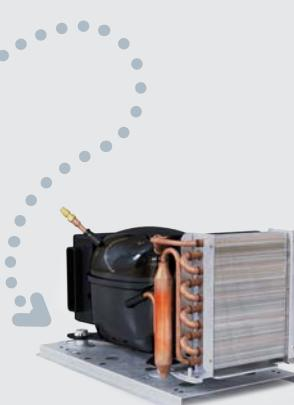
The remutable external cooling unit (In models with external cooling unit) offers added available volume inside the refrigerator. In addition, it expands the installation possibilities in terms of functionality, efficiency and soundproofing.
